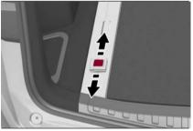
Adjustable Anchor Loop — If Equipped
