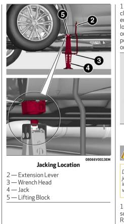
13. Rotate the extension lever clockwise until the round pin on the jack engages in the hole in the lifting block located about six inches (15 cm) from the outside edge of the body. The lifting points are marked by triangles  $\bigtriangledown$  visible on the plastic body panel.
