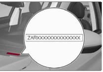
10016V0001EM Vehicle Identification Number This number is also stamped on the chassis near the front left shock absorber and can be seen by opening the engine compartment hood.
