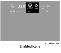
Setting a speed activates the system. The display shows the icon in green with the set speed.
