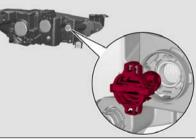
08026V0007EM Bulb/Connector 4. Remove the bulb by sliding it off the bulb holder.
