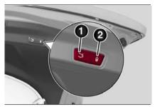
O4056V0055EM Power Liftgate/Lock Switches
