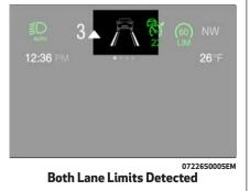
When lane limits are detected, the system is ready to provide indications in case the driver unintentionally leaves the lane (turn signal not activated). As the Lane Departure Warning system detects the lane limits while the vehicle is in motion, it will adjust the display accordingly (from white to yellow and yellow to white, and increase their thickness).
