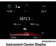
To reset the values, push and hold down the MENU button on the windshield wiper stalk.
