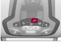
0404650002EM Volumetric/Anti-Lift Protection Button
